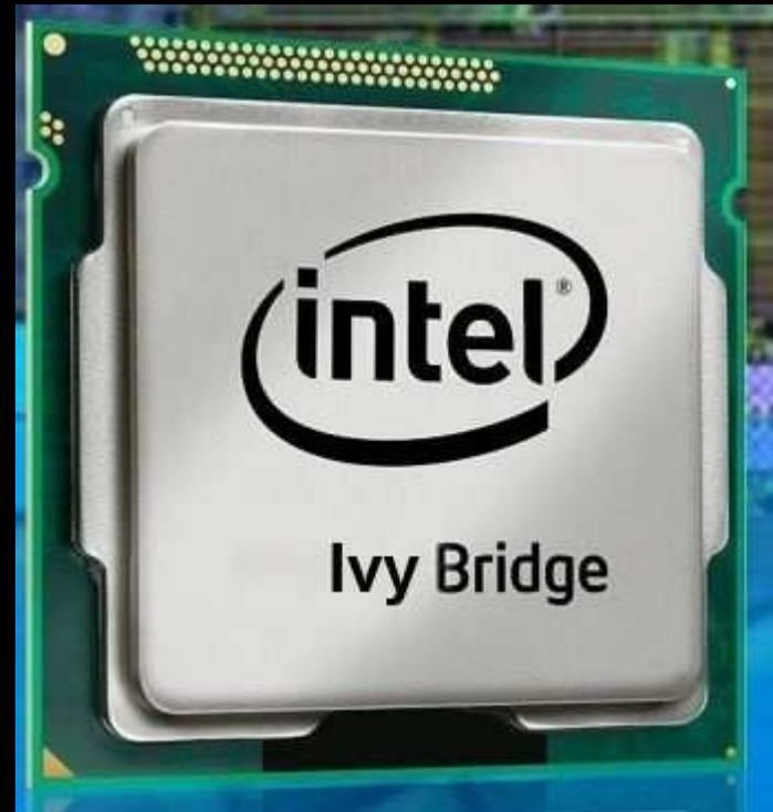
INTEL Ivy Bridge Central Processing Unit (chip fabricated by photolithography - 22 nm technology; 1,4 billion of transistors)
