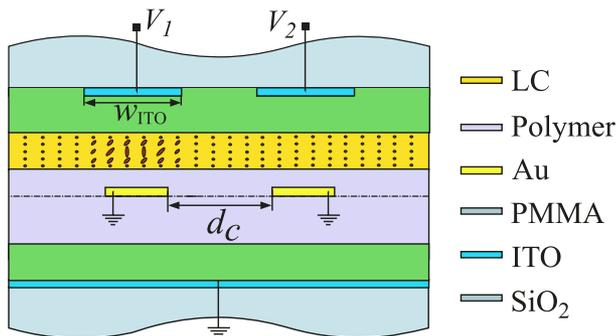
Two LC-LRSPP waveguides are side-coupled: individually addressed by voltages  $V_1$  and  $V_2$
