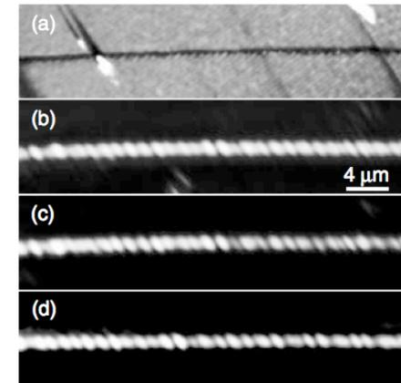
FIG. 4. Grayscale (a) topographical and near-field optical images ( $36 \times 9 \mu\text{m}^2$ ) taken with groove N2 at  $\lambda \cong$  (b) 1.44, (c) 1.5, and (d) 1.57  $\mu\text{m}$ . The CPP propagation is from left to right.
