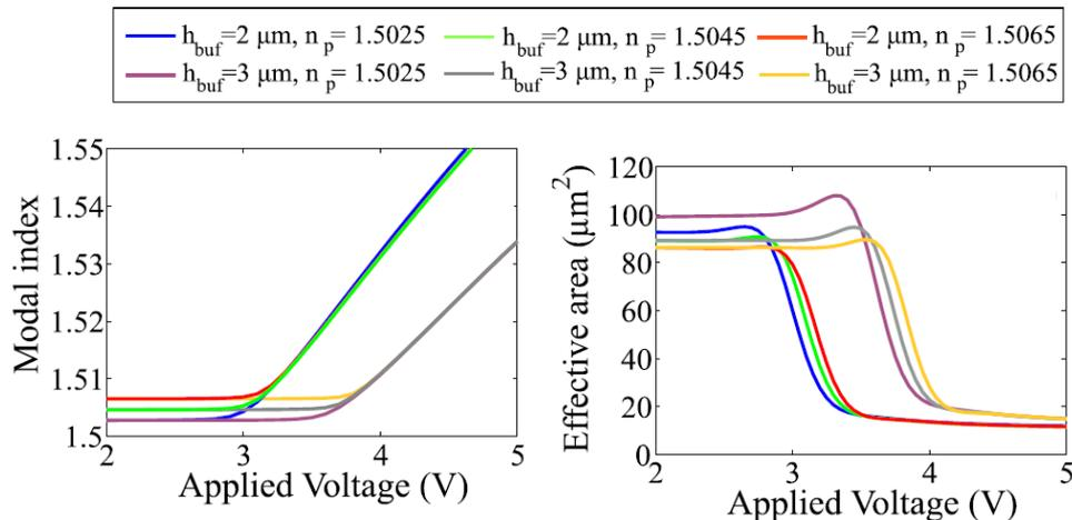
Above the LC switching threshold light escapes into the high-tilt LC-zone. Further increase of voltage raises the LC-waveguide index and reduces modal area, enhancing field confinement.
