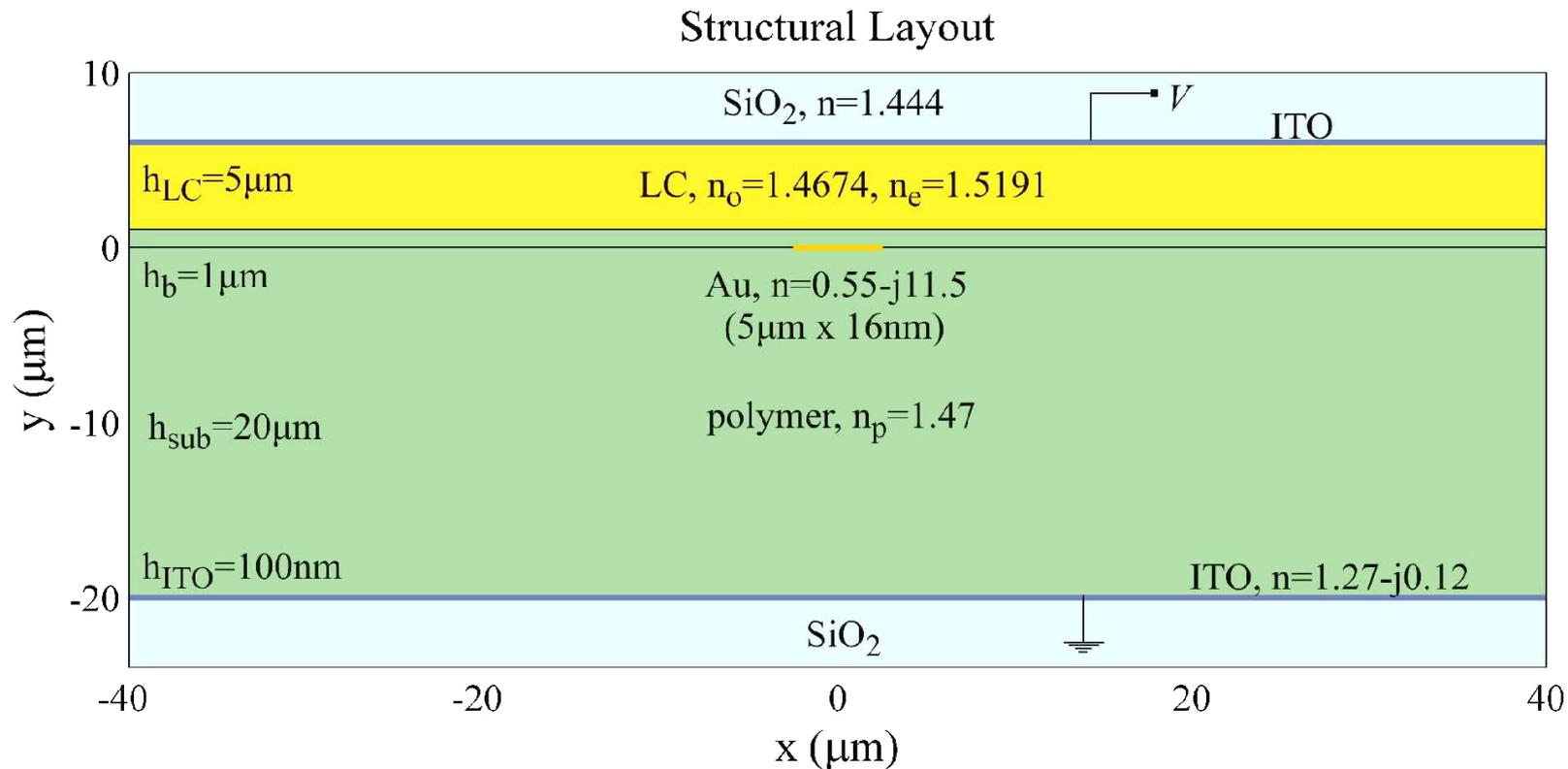
Light is initially confined in the bottom cladding
