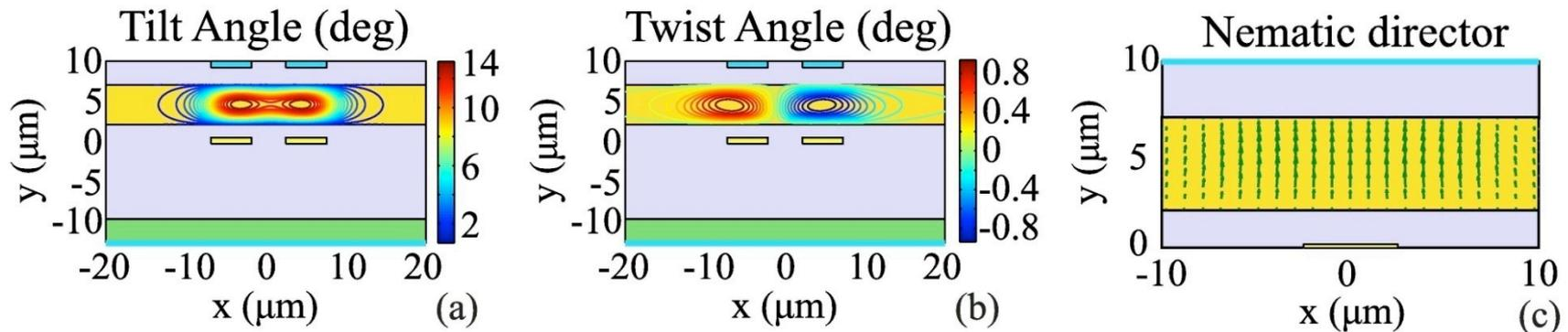
By raising the applied voltage  $V$  the supermodes of the directional coupler are no longer LR-SPP modes, but hybrid LRSPP-LC ones.
