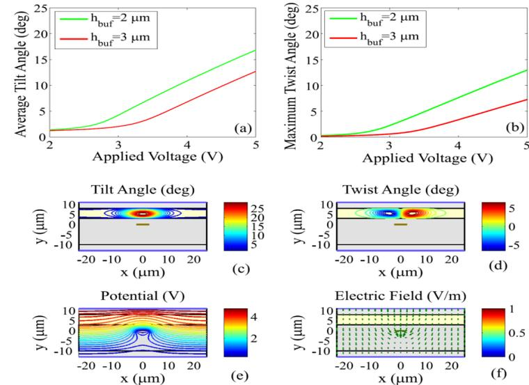
Figure 5: (a) Average tilt and (b) maximum twist angle calculated in the applied voltage range  $2 < V < 5$  V for two values of the buffer layer thickness of the waveguide LR2. (c-f) Tilt, twist, electrostatic potential, and electric field profiles at  $V = 5$  V for  $h_{buf} = 3$   $\mu\text{m}$ . A high-tilt zone is formed above the grounded metal stripe.
