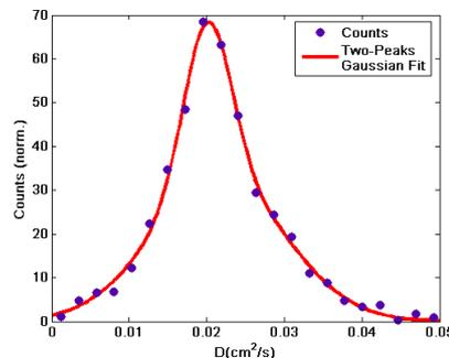
**Fig. 2:** Histogram of the thermal diffusivity.
