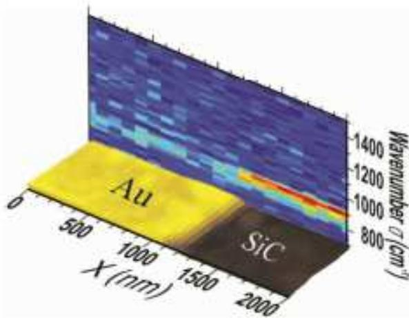
Fig. 1: Hyperspectral TRSTM line scan. Near-field thermal emission spectra are recorded each 100 nm along a straight line crossing a boundary between SiC and Au. A quasi-monochromatic near-field thermal emission is observed on SiC due to the contribution of surface phonon-polaritons [5].
