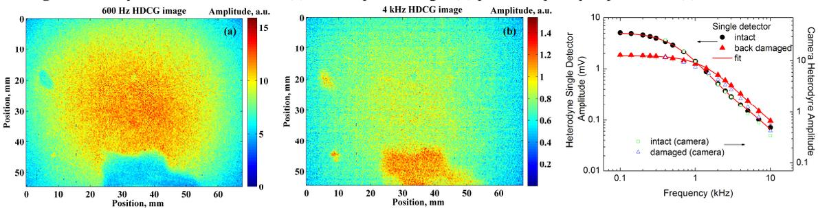
Fig. 2: Heterodyne LIC of the same wafer (a) at 600 Hz; (b) at 4 kHz; (c) amplitude-frequency dependence. Notice the amplitude contrast inversion at high frequencies.
