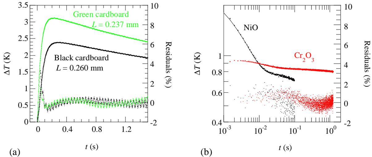
**Fig. 1.** Results obtained from both front and back flash methods. Experimental results are shown by dots and continuous lines represent the curve-fittings obtained from the models. (a) Classical (back configuration) flash method results in cardboards. (b) Front face configuration results for magnetic oxides that are semitransparent to IR wavelengths.
