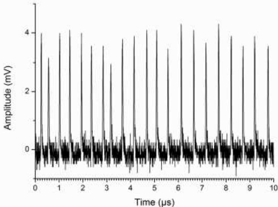
Fig. 1: Direct probe detection of a nanobubble under constant heating just above the boiling threshold. The signal shows quasi-periodic bursting behavior, with each burst lasting for a few tens of ns.
