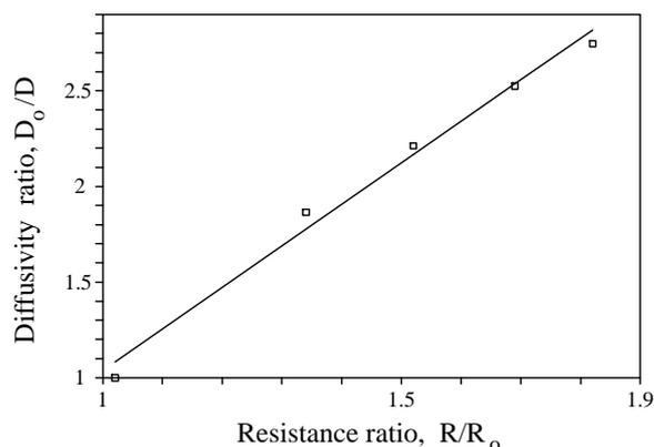
Figs.1 exp.setup: Fig.2: correlation curve between the diffusivity ratio and the electrical resistance ratio
