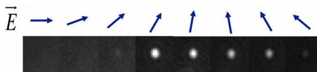
**Fig. 1.** Polarization-dependent optical backscattering response of a single irradiated gold nanorod
