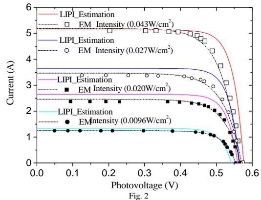
Fig. 1 The determination of a mc-Si solar cell power dissipated by using LIT. Fig. 2 The estimation of current-voltage characteristic of the solar cell using contactless LIC
