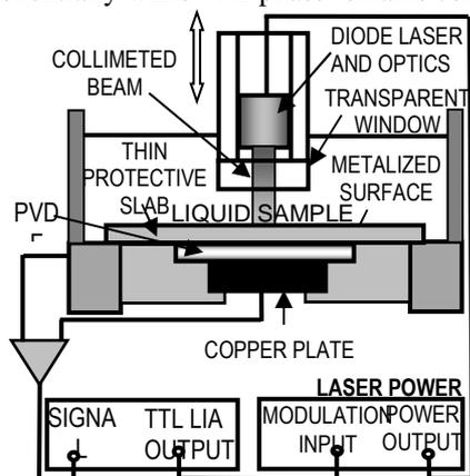
**Fig. 1** Cross section of the Photopyroelectric setup.
