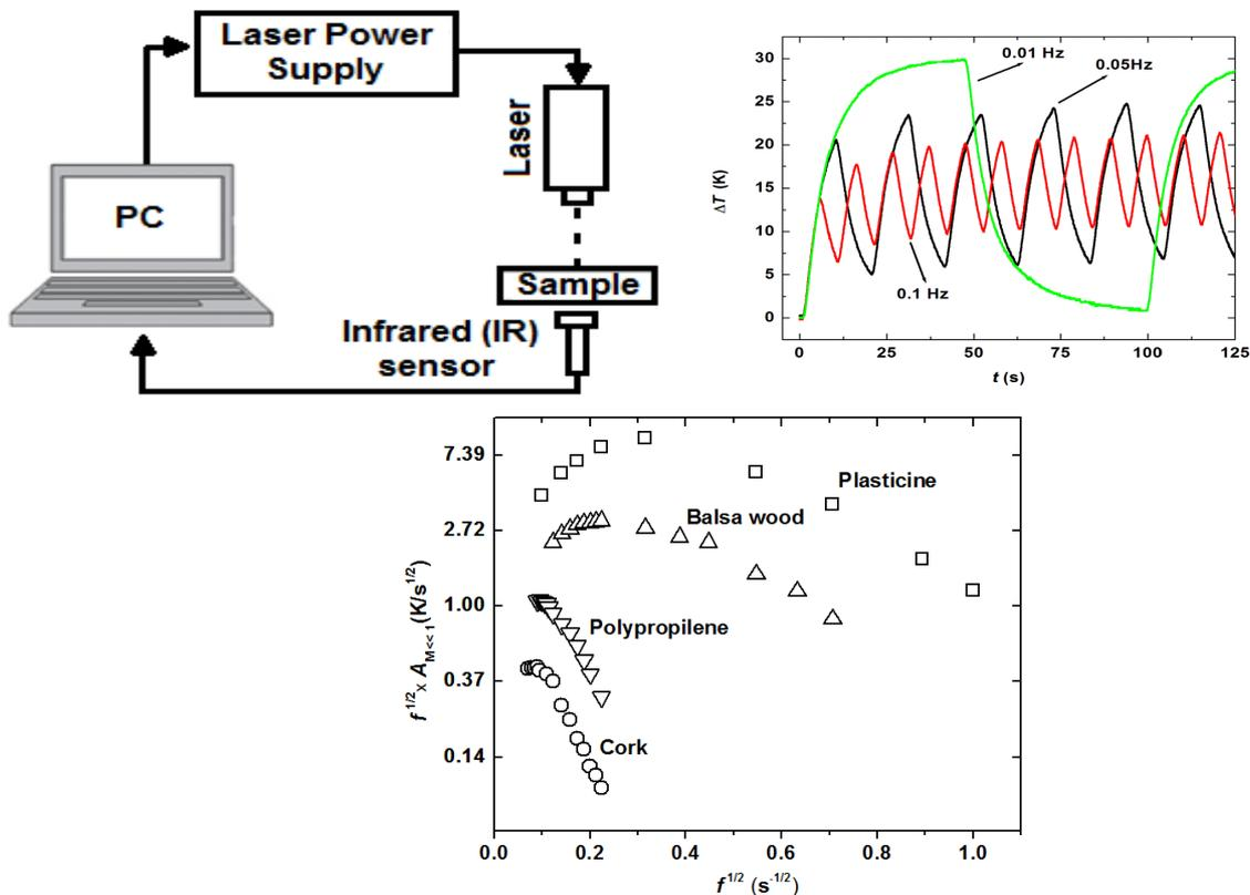
**Figure:** Top left: experimental setup. Top right: typical IR signals. Bottom: frequency dependence of IR radiometry signals of different samples, containing features due to convective and radiative heat losses.
