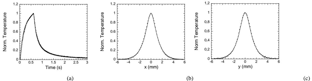
Fig. 1: Experimental (dots) and fitted (continuous line) temporal evolution of the temperature at the center of the thermogram (a), and central profiles obtained at the end of a 300 ms burst perpendicular to the crack (b) and along the crack (c) corresponding to a 1 by 1 mm square vertical crack buried 0.6 mm below the sample surface.
