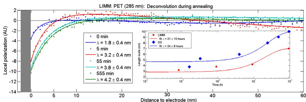
**Fig. 1:** Pyroelectric surface profiles on PET thin films measured by LIMM as function of sample annealing time.
