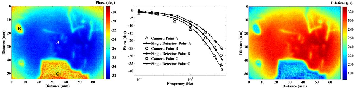
Fig. 1: Homodyne LIC of a c-Si wafer (a) 300 Hz phase image; (b) phase-frequency dependence; (c) effective lifetime image
