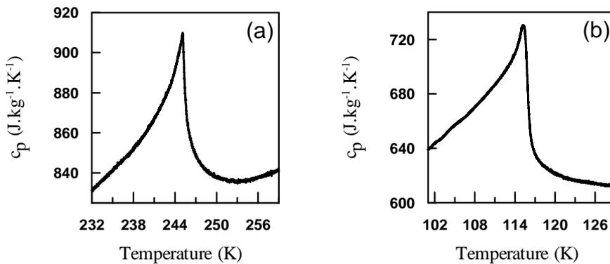
Fig. 1: Specific heat for  $\text{KNiF}_3$  (a) and  $\text{KCoF}_3$  (b) in the vicinity of the magnetic transition
