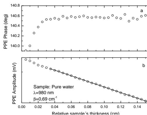
**Fig. 2** Photopyroelectric (PPE) signal, as a function of the sample's thickness, for pure water. a. PPE phase. b. PPE amplitude. The continuous line in b is the best linear fit for obtaining the optical absorption coefficient.
