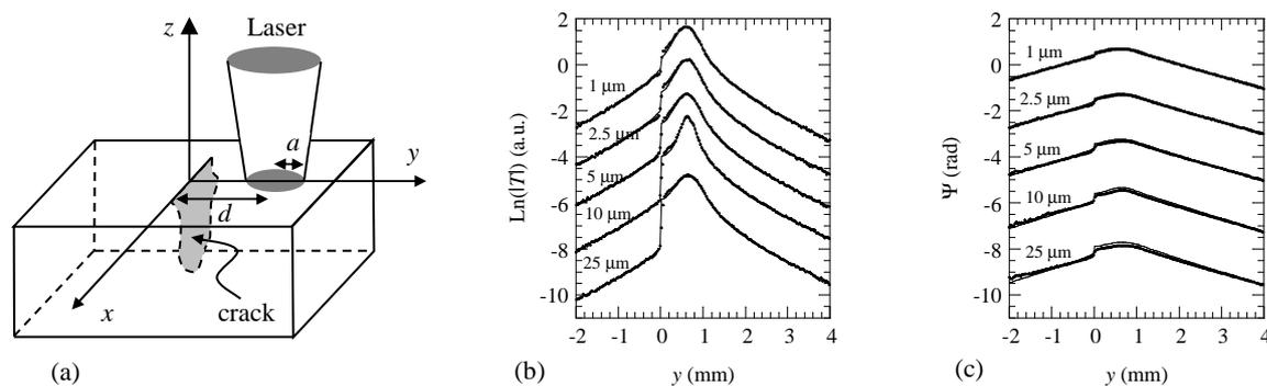
**Fig. 1:** (a) Diagram of the vertical crack of arbitrary shape. (b) Experimental natural logarithm of the surface temperature amplitude and (c) phase profiles along the  $y$  axis for several crack widths, for infinite cracks. Dots correspond to experimental data and continuous lines to the fit to theory (for the sake of clarity data have been shifted vertically).
