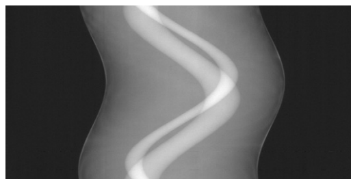
Fig. 13. Sinogram below iodine K-edge of a cylindrical phantom of a cylindrical phantom.
