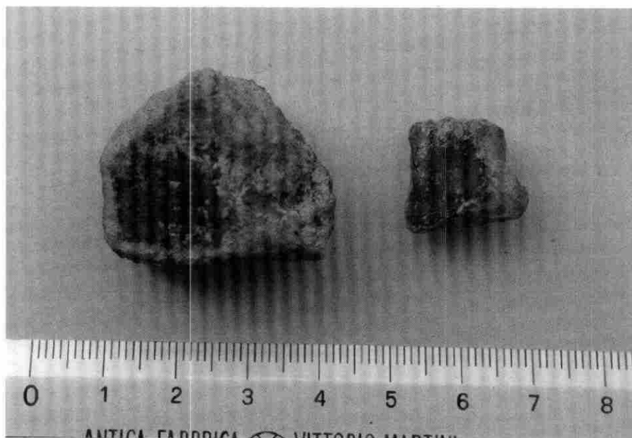
Fig. 8. A block of litharge, AS2 846 (left) and a piece of a copper ingot, ASE 6 (right) (see also Fig. 6, 19 and 21).
