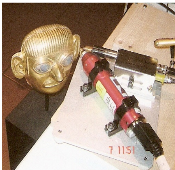
Fig. 2 Experimental set-up, showing, on the left, the Eclipse II X-ray tube (collimated with a brass cylinder), with Ag-anode and working at 30 kV, 100 \mu A maximum voltage and current, and the Si-PIN detector (also collimated with a brass cylinder), during measurements on the golden mask, in the Museum “Tumbas Reales de Sipán”. A typical measurement takes 50-200 s, depending on the geometry and object composition.
