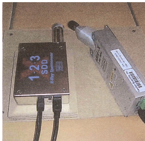
Fig. 3 EDXRF-portable equipment, composed of a Si-drift detector (~450 \mu m thickness, 7 mm 2 area and 140 eV energy-resolution at 5.9 keV) and a X-Ray tube (40 kV, 100 \mu A maximum voltage and current, and Ag-anode). Electronics, including bias supply and MCA are in the case of tube and detector.
