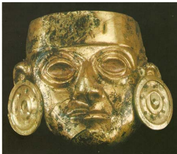
Fig. 17 Mask made of gilded copper from the tomb n. 3 of “tumbas reales de Sipán” Areas relatively free from Cu-compounds have been analyzed. A gilding thickness of \sim 0.6 \mu\text{m} was determined.
