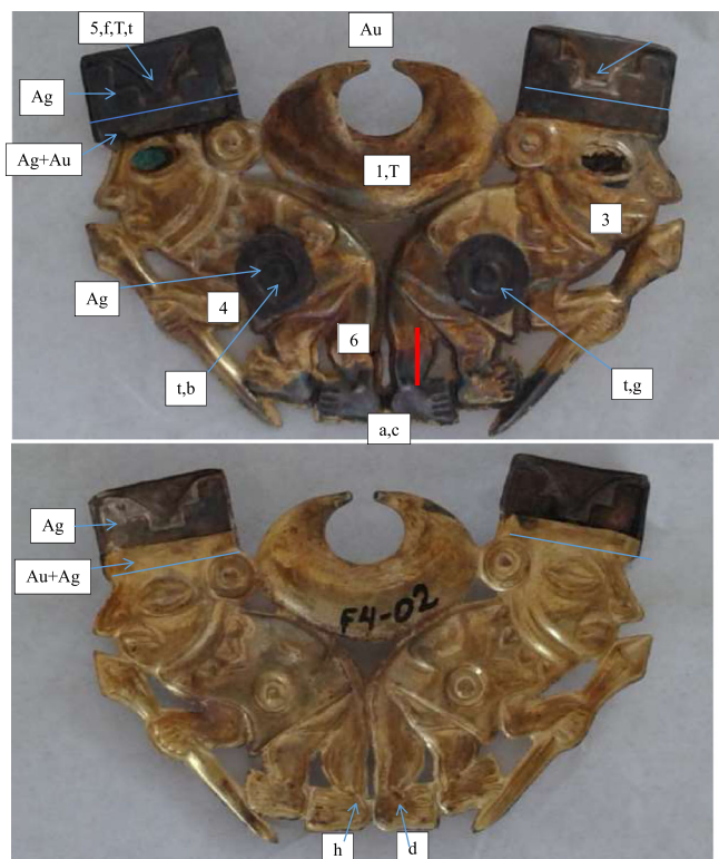
Figure 15. Front and rear side of the nose decoration PACEB-F4-0002. It is composed of a body on laminated gold alloy with two shields (on the front side) and two huts on almost pure silver superimposed and glued. T and t indicate areas where transmission measurements were carried out, numbers 1–6 and a–h EDXRF-measurements carried out in 2014 and 2015, respectively. The red vertical line indicates the radiographic profile shown in Fig. 20. Gold alloy composition: Au = 74.5\% , Ag = 19.5\% , Cu = 5.5\% . Silver alloy composition: Ag = 99.2\% , Cu = 0.02\% , Au = 0.8\% .
