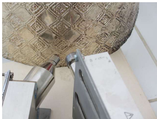
Figure 4. Energy-dispersive X-ray fluorescence portable equipment, composed of a Si-drift detector (on the right; 123SDD: 450- \mu m thickness, 7-mm 2 area, and 125-eV energy-resolution at 5.9 keV) and a Ag-anode X-ray tube (40 kV, 100- \mu A maximum voltage and current) (38). Electronics including bias supply and Multi-Channel Analyzer (MCA) are in the case of the detector; X-ray tube bias supply is in the case of the X-ray tube. A typical measurement takes 50–100 s. The energy-dispersive X-ray fluorescence-equipment is analyzing the crown PACEB-F4-00069.
