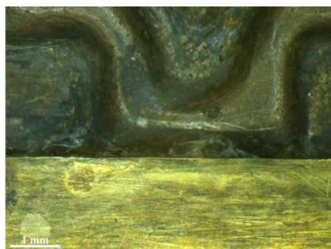
Figure 23. Optical microscopy image of the back side of the nose decoration PACEB-F4-0002 (Fig. 15), which shows residual material at the interface between gold and silver laminae.
