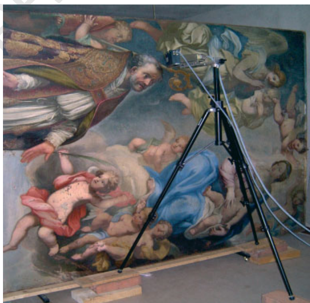
Figure 8 Portable EDXRF equipment for analysis of pigments in paintings and frescos. It is composed of a 50-kV, 1-mA X-ray tube and an Si-drift detector.
