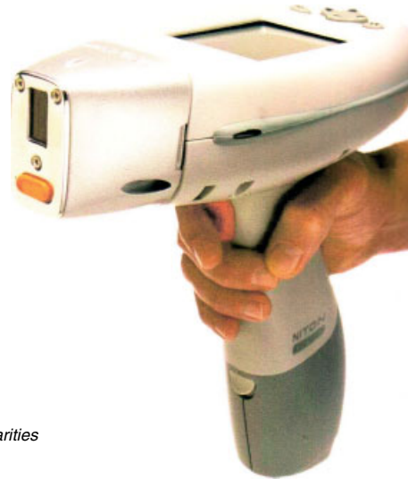
Figure 5 Typical modern Thermo Scientific Niton handheld EDXRF-analyzer. (With permission of Thermo Fisher Scientific.)
