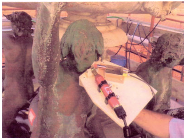
Figure 9 Portable EDXRF equipment for analysis of bronzes and gold alloys. It is composed of an Eclipse II X-ray tube (30 kV, 100 \mu A) and an Si-PIN detector.
