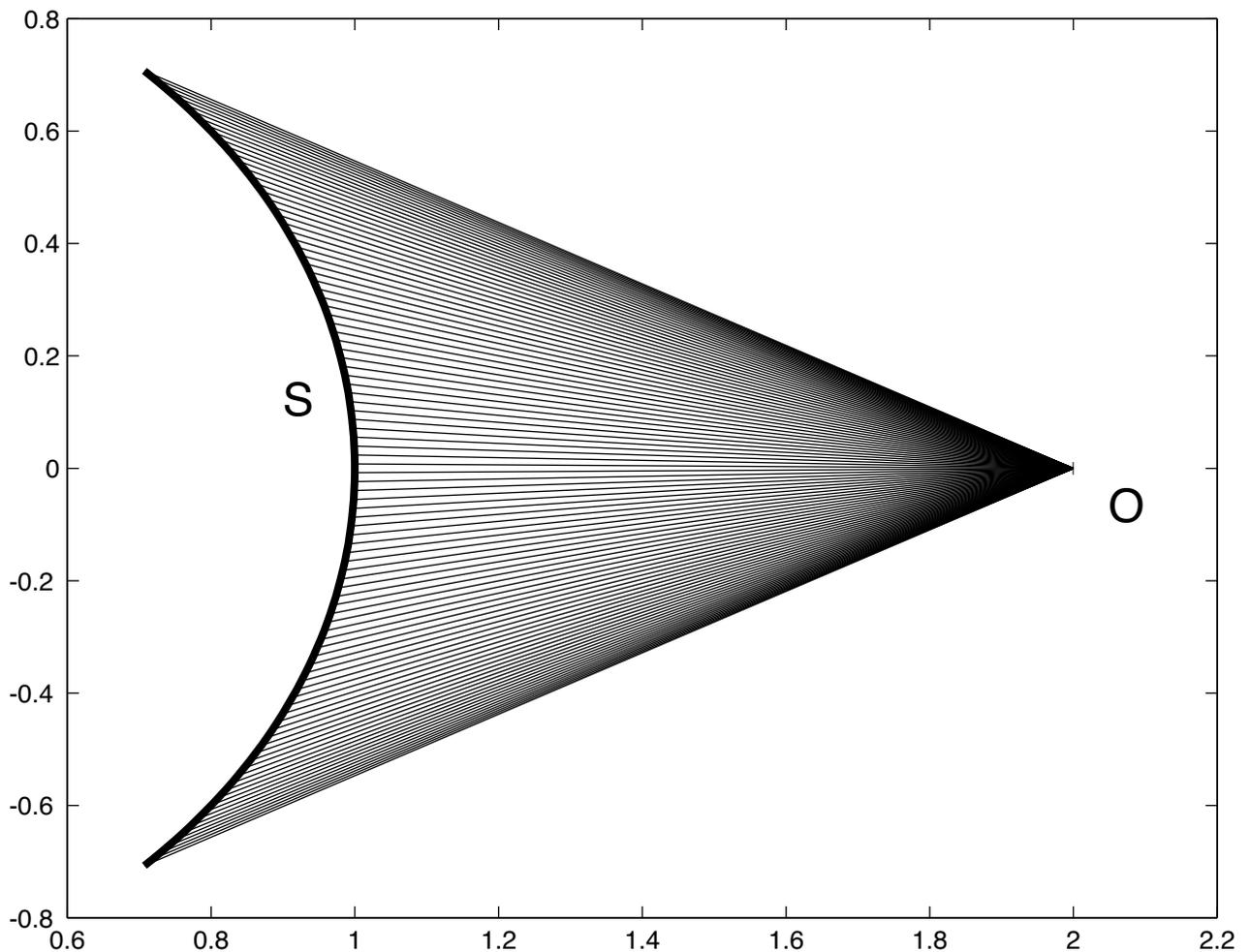
Optimal distribution of a [conductor](#) for heat sources  $f = \mathcal{H}^1 \llcorner S - L\delta_O$ .
