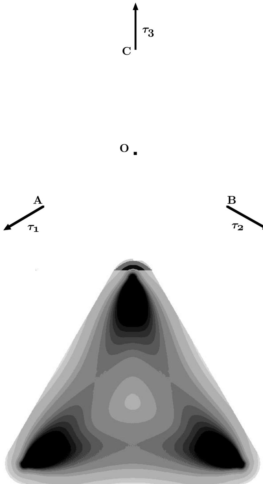
Optimal distribution of an [elastic material](#) when the forces are as above.
