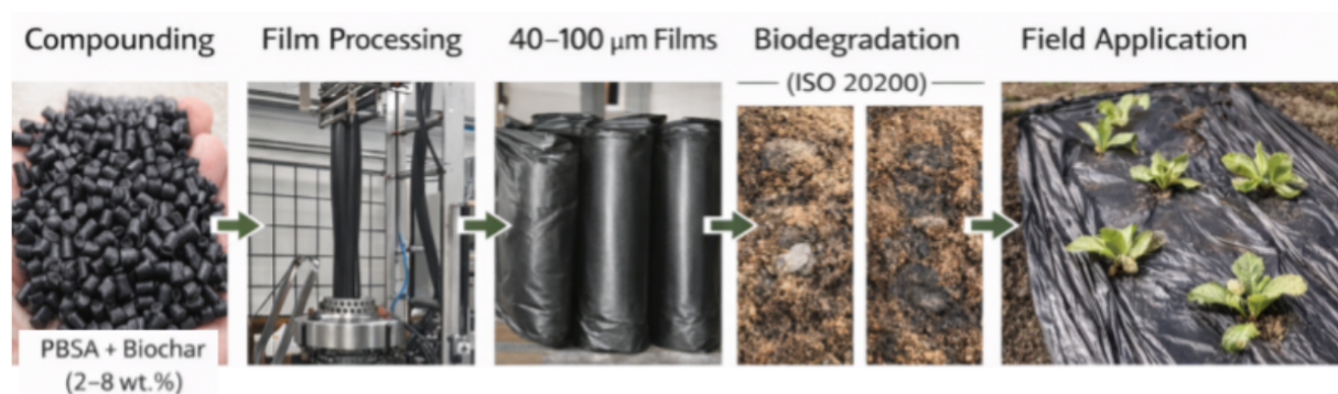
Figure 1. Processing workflow of PBSA/biochar mulch films.
