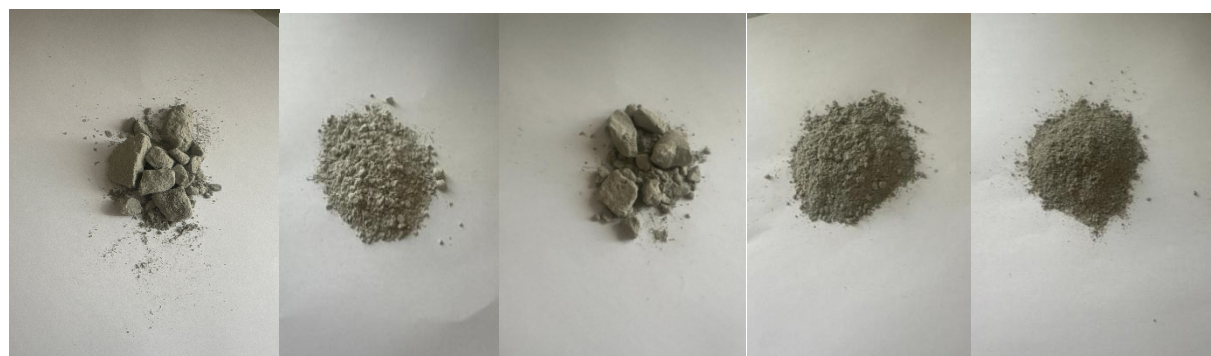
Figure 1. Sawing sludges images.
