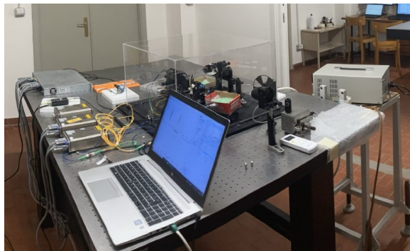
Figura 2 Spectroscopy/imaging system based on Photoconductive antennas and DFB fiber-coupled IR laser.
