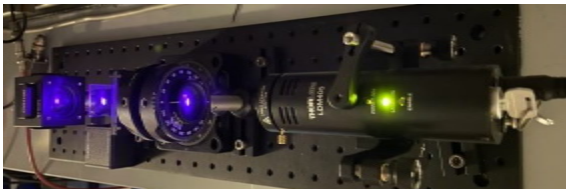
Figure 1. Set up for the measurements of the fluorescence detected circular dichroism on molecules deposited on nanostructures, excited by UV light.
