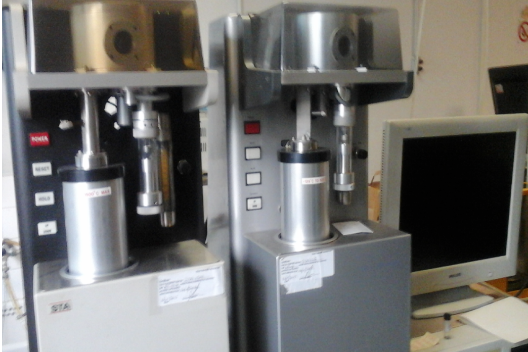
Figure 1) Stanton Redcroft Simultaneous Thermogravimetry and Differential Thermal Analysis (TG/DTA) equipments (STA 1500 and STA 625 models on the left and right, respectively)
