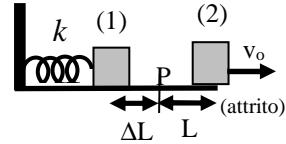
$$\text{Energia meccanica in (2)} \quad E_2 = \frac{1}{2} m \cdot v_0^2$$
