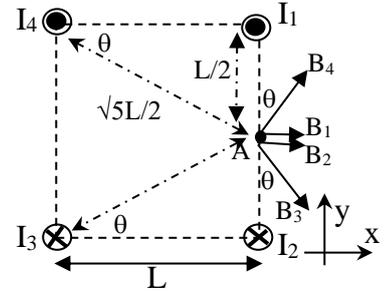
lungo  $x$   $B_{3,x} = B_{4,x} = \frac{\mu_0(2I)}{2\pi(\sqrt{5}L/2)} \sin\theta = \frac{\mu_0(2I)}{2\pi(\sqrt{5}L/2)} \frac{L/2}{\sqrt{5}L/2} = \frac{2}{5} \frac{\mu_0 I}{\pi L}$
