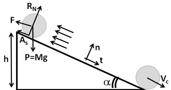
$$A_s r = I_c \frac{d\omega}{dt} = I_c \frac{a_c}{r} \quad \text{da cui} \quad A_s = \frac{I_c}{r^2} a_c \quad (2)$$
