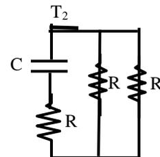
$$\text{Imponendo } q(\Delta t_2) = q_0 \text{ si ottiene } \Delta t_2 = \tau_2 \ln \left( \frac{q(\Delta t_1)}{q_0} \right) = 19 \text{ ms}$$
