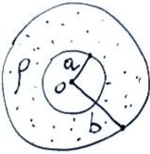
$$V(0) - V(A) = \int_0^a \vec{E}_0^{\text{INT}} \cdot d\vec{l} + \int_a^b \vec{E} \cdot d\vec{l} + \int_b^{2b} \vec{E}_0^{\text{EXT}} \cdot d\vec{l}$$
