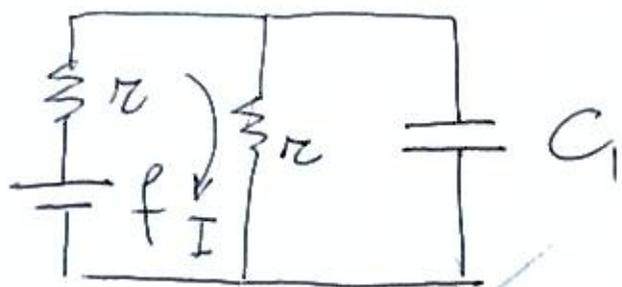
$$Q_1^0 = C_1 \Delta V_{C_1} = C_1 \frac{f}{2}$$
