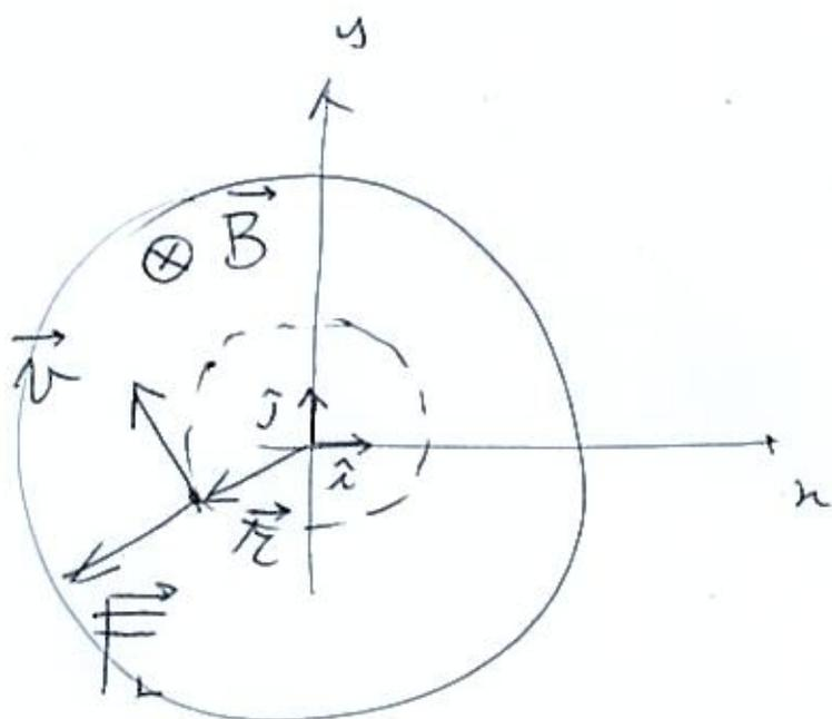
$$\frac{\vec{F}_L}{q} = \vec{E} = \vec{v} \times \vec{B} = \omega B \vec{r}$$
