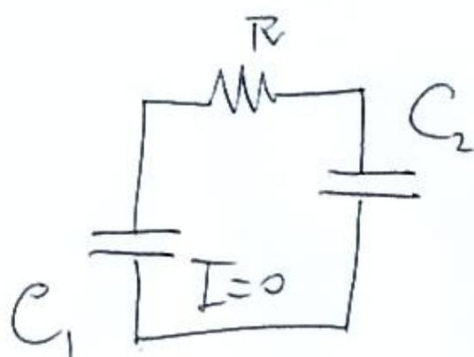
$$\left\{ \begin{array}{l} Q_1^\infty + Q_2^\infty = Q_1^0 \\ \text{ma:} \\ \frac{Q_1^\infty}{C_1} = \frac{Q_2^\infty}{C_2} \end{array} \right.$$
