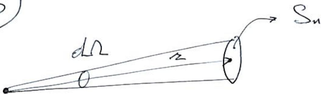
$$I = \frac{F_{\text{eff}}^2}{Z_0} \quad ; \quad \Omega = \frac{S_n}{r^2}$$
