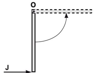
$$\frac{1}{2} I_O \omega^2 = mg \frac{L}{2} \quad \Rightarrow \quad \omega = \sqrt{\frac{3g}{L}} = 5.4 \text{ rad s}^{-1} \quad \Rightarrow \quad J = 1.8 \text{ N s}$$
