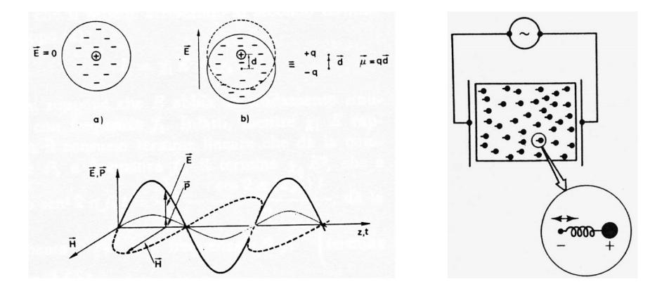
Origin of the dielectric response – Microscopic model – Linear Case
