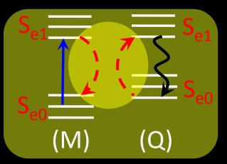
If the quencher is not luminescent it can dissipate the energy through non-radiative paths
