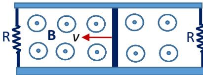
$$\begin{aligned} \Phi &= B S(t) \\ S(t) &= l x(t) \\ f_{em} &= -\frac{d\Phi}{dt} = -Blv \end{aligned}$$
