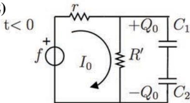
$$C_s = \frac{C_1 C_2}{C_1 + C_2} = \frac{C_1}{2} \quad Q_0 = C_s R' I_0 = \frac{C_1 R' f}{2 r + R'}$$
