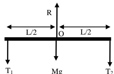
$$\begin{cases} F^{ext} = R - T_2 - T_1 - Mg = 0 \\ M^{ext} = M_{T_1} + M_{T_2} = +T_1\left(\frac{L}{2}\right) - T_2\left(\frac{L}{2}\right) = 0 \end{cases}$$
