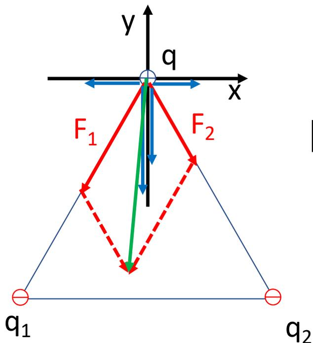
$$|\vec{F}_1| = \frac{q_1 q}{4\pi\epsilon_0 L^2} \quad F_{1x} = \frac{q_1 q}{4\pi\epsilon_0 L^2}(-\sin 30^\circ) \quad F_{1y} = \frac{q_1 q}{4\pi\epsilon_0 L^2}(-\cos 30^\circ)$$
