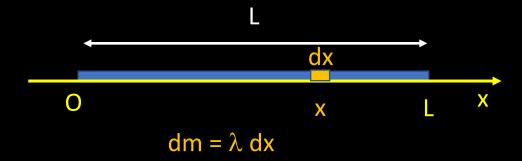
$$x_{CM} = \frac{\int_{L} x \, dm}{m} = \frac{\int_{0}^{L} x \, \lambda \, dx}{m} = \lambda \frac{\int_{0}^{L} x \, dx}{m} = \frac{m}{L} \frac{\frac{1}{2}L^{2}}{m} = \frac{L}{2}$$
