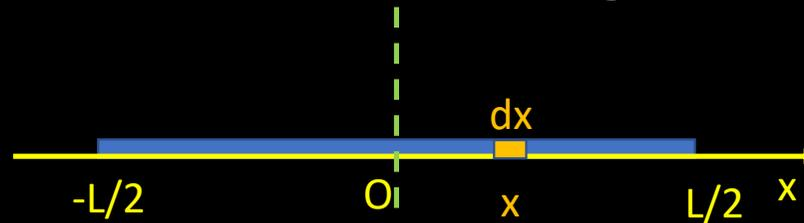
$$I = \int_V r^2 dm \rightarrow I = \int_{-L/2}^{+L/2} x^2 \lambda dx = \frac{m}{L} \int_{-L/2}^{+L/2} x^2 dx = \frac{m}{L} \left[ \frac{(L/2)^3}{3} - \frac{(-L/2)^3}{3} \right] = m \frac{L^2}{12}$$
