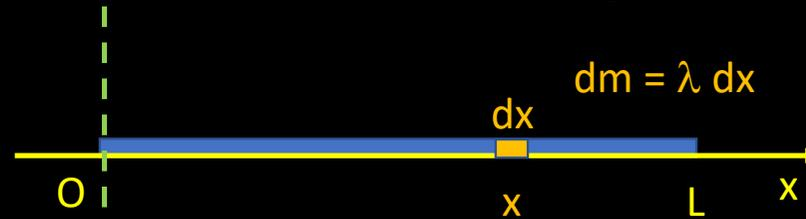
$$I = \int_V r^2 dm \rightarrow I = \int_0^L x^2 \lambda dx = \lambda \int_0^L x^2 dx = \frac{m}{L} \int_0^L x^2 dx = \frac{m}{L} \left[ \frac{L^3}{3} - \frac{0}{3} \right] = m \frac{L^2}{3}$$
