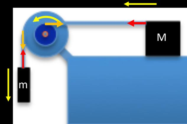
$$mg - F_1 = ma = m\alpha 2R \rightarrow F_1 = mg - 2 m\alpha R$$
