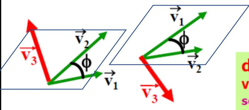
$$|\vec{v}_1 \times \vec{v}_2| = v_1 v_2 \sin(\phi)$$
