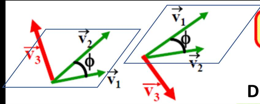
$$|\vec{v}_1 \wedge \vec{v}_2| = v_1 v_2 \text{ sen } \phi$$
