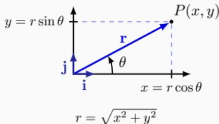
$$r = \sqrt{x^2 + y^2} = 17,3 \text{ m} \qquad \tan \theta = \frac{8,7 \text{ m}}{15,0 \text{ m}} \Rightarrow \theta = 30^\circ.$$
