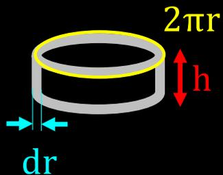
$$U = \int_{\tau} u \, d\tau = \int_{R_1}^{R_2} \frac{1}{2} \mu_0 \left(\frac{I}{2\pi r}\right)^2 2\pi r h \, dr = \frac{1}{2} \frac{\mu_0 h I^2}{2\pi} \ln\left(\frac{R_2}{R_1}\right)$$
