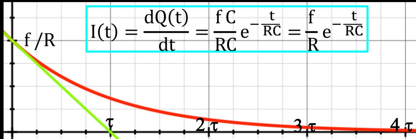
$$I(t) = \frac{dQ(t)}{dt} = \frac{f C}{RC} e^{-\frac{t}{RC}} = \frac{f}{R} e^{-\frac{t}{RC}}$$
