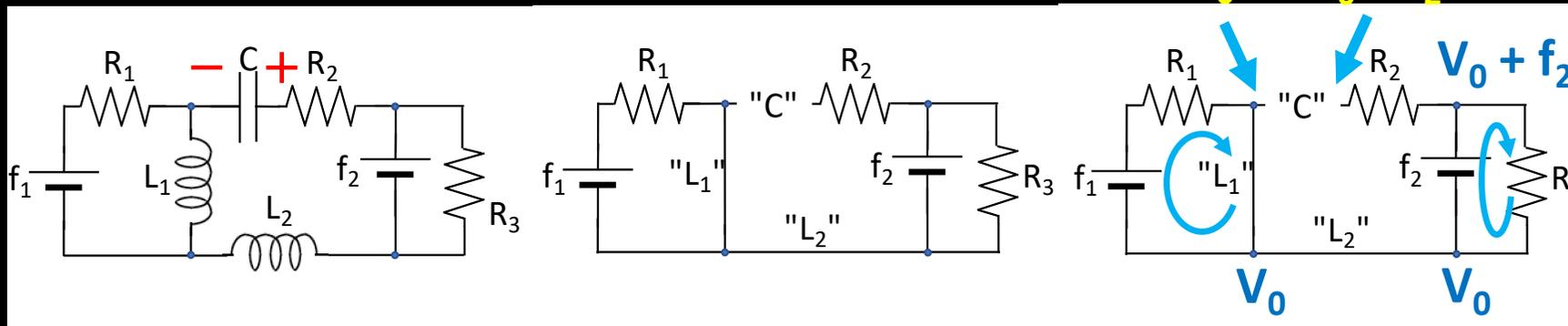
$$I_{R_1} = f_1/R_1 = 5 \text{ V}/100 \ \Omega = 0,05 \text{ A}$$
