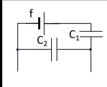
$$C_S = C_1 C_2 / (C_1 + C_2) = C^2 / 2C = C/2$$
