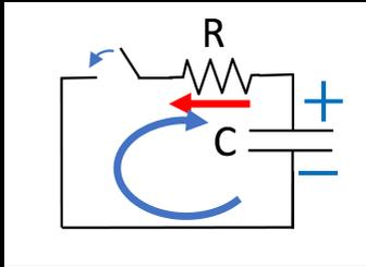
$$\Delta V_C(0^+) = \Delta V_C(0^-) = \Delta V_0 = \frac{Q_0}{C} \neq 0$$
