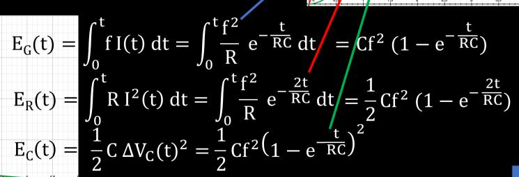
$$\int_{0}^{t} R I^{2}(t) dt = \int_{0}^{t} \frac{f^{2}}{R} e^{-\frac{2t}{RC}} dt = \frac{1}{2} Cf^{2} (1 - e^{-\frac{2t}{RC}})$$
