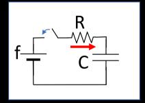
$$I(t) = \frac{dQ(t)}{dt} = \frac{fC}{RC}e^{-\frac{t}{RC}} = \frac{f}{R}e^{-\frac{t}{RC}}$$
