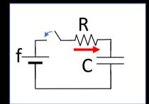
$$I(t) = \frac{dQ(t)}{dt} = \frac{fC}{RC}e^{-\frac{t}{RC}} = \frac{f}{R}e^{-\frac{t}{RC}}$$
