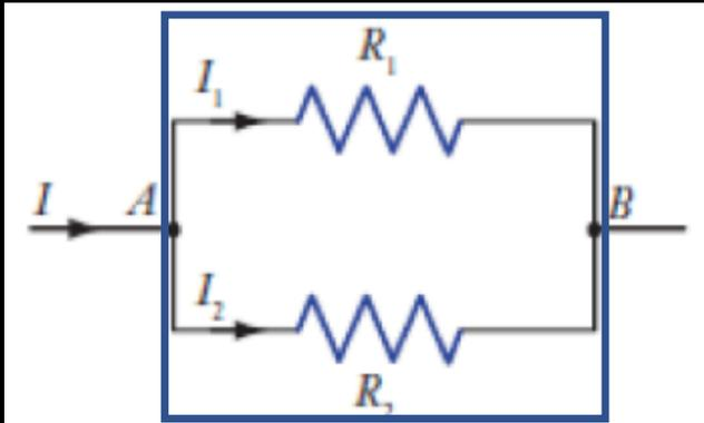
$$\frac{1}{R_p} = \frac{I}{\Delta V_{AB}} = \frac{I_1 + I_2}{\Delta V_{AB}} = \frac{I_1}{\Delta V_{AB}} + \frac{I_2}{\Delta V_{AB}} = \frac{1}{R_1} + \frac{1}{R_2} = \frac{R_1 + R_2}{R_1 R_2}$$
