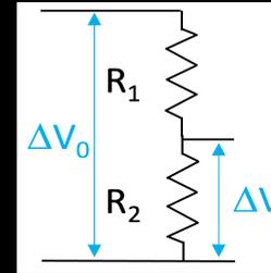
$$\Delta V = \Delta V_0 \frac{R_2}{R_1 + R_2}$$
