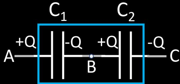
$$\frac{1}{C_S} = \frac{\Delta V_{AC}}{Q} = \frac{\Delta V_{AB} + \Delta V_{BC}}{Q} = \frac{\Delta V_{AB}}{Q} + \frac{\Delta V_{BC}}{Q} = \frac{1}{C_1} + \frac{1}{C_2} = \frac{C_1 + C_2}{C_1 C_2}$$
