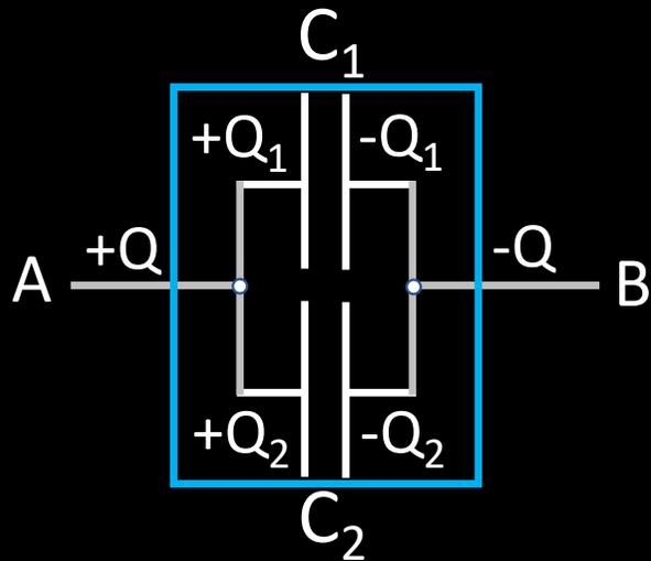
$$C_P = \frac{Q}{\Delta V_{AB}} = \frac{Q_1 + Q_2}{\Delta V_{AB}} = \frac{Q_1}{\Delta V_{AB}} + \frac{Q_2}{\Delta V_{AB}} = C_1 + C_2$$
