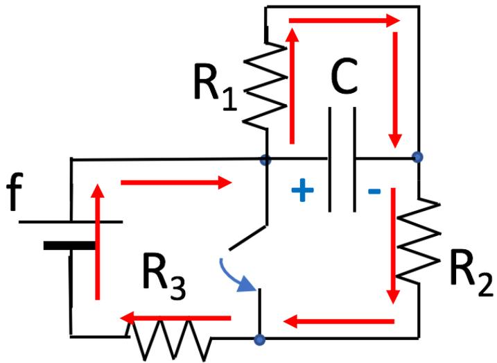
$$I = f / (R_1 + R_2 + R_3)$$
