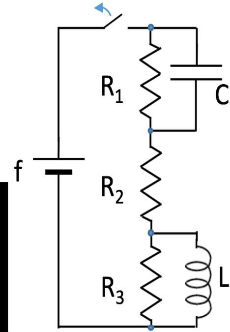
$$\Delta V_C(0) = R_1 I = R_1 f / (R_1 + R_2) = 100 \times 6 / (100 + 100) = 3 \text{ V}$$
