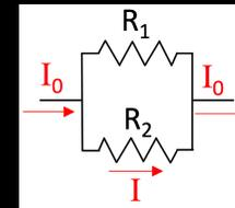
$$I = I_0 \frac{R_2}{R_1 + R_2}$$
