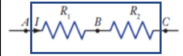
$$R_S = \frac{\Delta V_{AC}}{I} = \frac{\Delta V_{AB} + \Delta V_{BC}}{I} = \frac{\Delta V_{AB}}{I} + \frac{\Delta V_{BC}}{I} = R_1 + R_2$$
