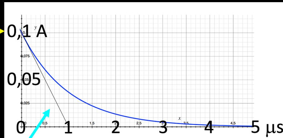
$$\tau = RC = 1 \mu\text{s} \rightarrow R = 1 \mu\text{s} / 20 \text{ nF} = 50 \Omega$$
