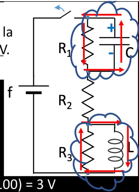
$$\Delta V_C(0) = R_1 I = R_1 f / (R_1 + R_2) = 100 \times 6 / (100 + 100) = 3 \text{ V}$$
