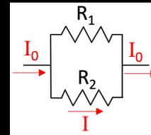
$$I = I_0 \frac{R_1}{R_1 + R_2}$$
