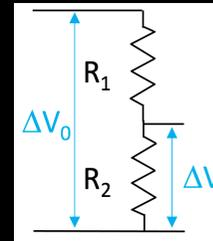
$$\Delta V = \Delta V_0 \frac{R_2}{R_1 + R_2}$$
