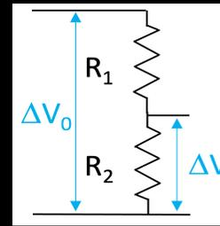
$$\Delta V = \Delta V_0 \frac{R_2}{R_1 + R_2}$$
