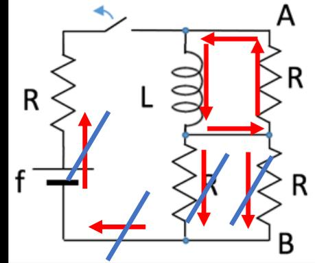
$$V_0 + f - RI - R_P I = V_0$$
