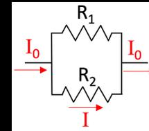
$$I = I_0 \frac{R_1}{R_1 + R_2}$$
