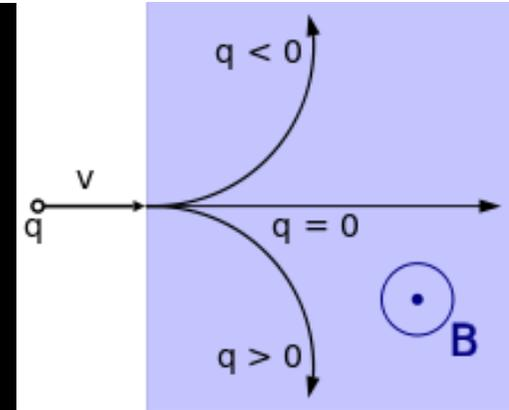
$$L = \int_{\gamma} \vec{F} \cdot d\vec{l} = \int_{\gamma} (q \vec{v} \times \vec{B}) \cdot \vec{v} dt = 0 \rightarrow |\vec{v}| = \text{costante}$$
