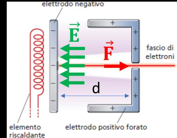
$$L = \int_{\gamma} \vec{F} \cdot d\vec{l} = \int_0^d F dl = \int_0^d eE dl = e E d = \frac{1}{2} m v_{\text{fin}}^2 - \frac{1}{2} m v_{\text{in}}^2 = \frac{1}{2} m v_{\text{fin}}^2$$
