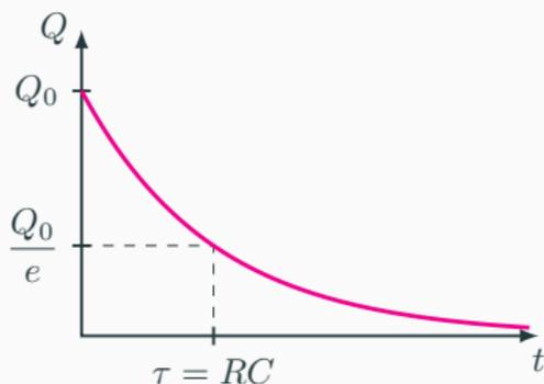
$$i = -\frac{dQ}{dt} = Q_0 \frac{1}{RC} e^{-\frac{t}{RC}} = \frac{V_0}{R} e^{-\frac{t}{RC}}$$
