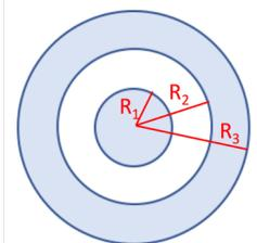
>>> soluzione:  $B(r < R_1) = \mu_0 I r / (2\pi R_1^2)$ ;  $B(R_2 > r > R_1) = \mu_0 I / (2\pi r)$ ;
