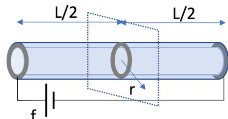
>>> soluzione:  $J = 5 \text{ A/mm}^2$ ;  $B(r < R_1) = 0$ ;  $B(R_1 < r < R_2) = \mu_0 J (r^2 - R_1^2) / (2r)$ ;  $B(r > R_2) = \mu_0 J (R_2^2 - R_1^2) / (2r)$
