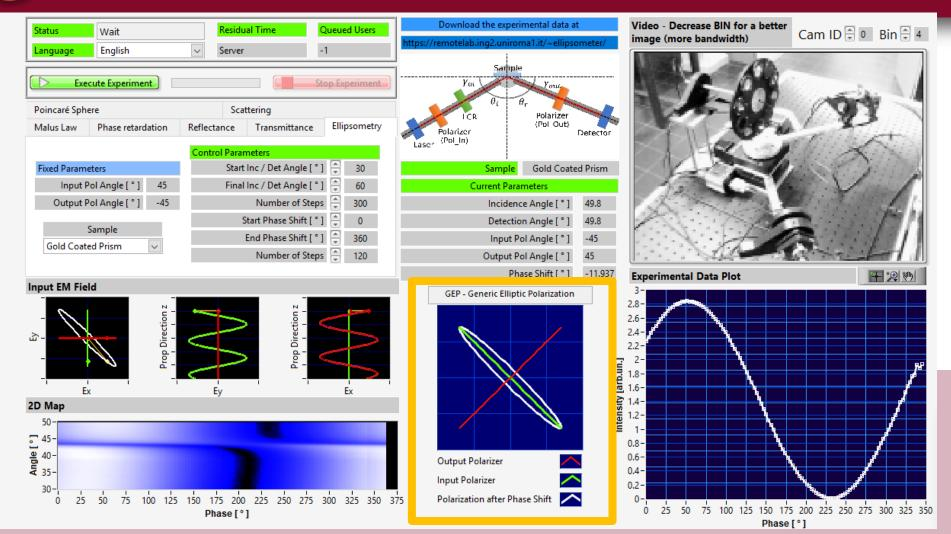
**Polarization Window** Shows the real time polarization state after the input polarizer, after the LCR cell and after the analyzer
