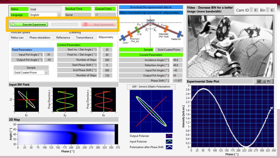
**Execute Window** Permits to launch and stop the measurement and displays a progression percentage bar
