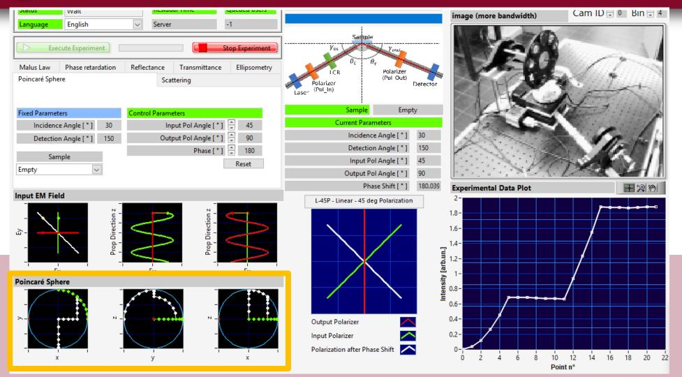
**Poncaré Window** Shows projections of the Poincaré sphere and the state after the input polarizer, after the LCR cell and after the analyzer
