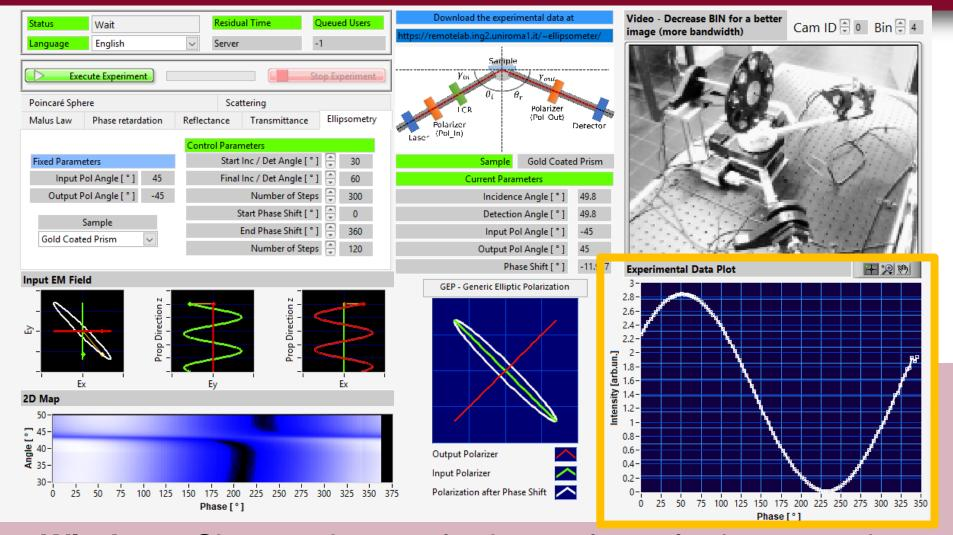
**Plot Window** Shows the real time plot of the experimental measurement in the operation mode chosen by the user
