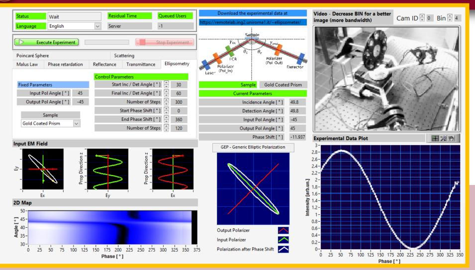
The GUI panel is characterized by several different windows dedicated to the control of the remote ellipsometer and to data flow
