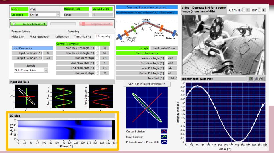
Map Window Shows a map of the experimental values for those experiments in which two control parameters are changed
