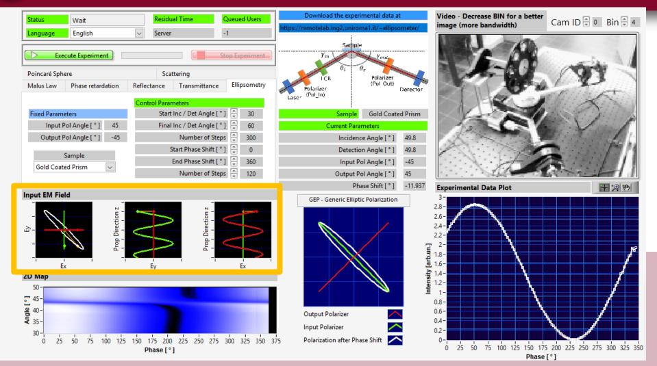
**Fields Window** Shows a simulation of the electromagnetic field illuminating the sample (after the LCR cell)
