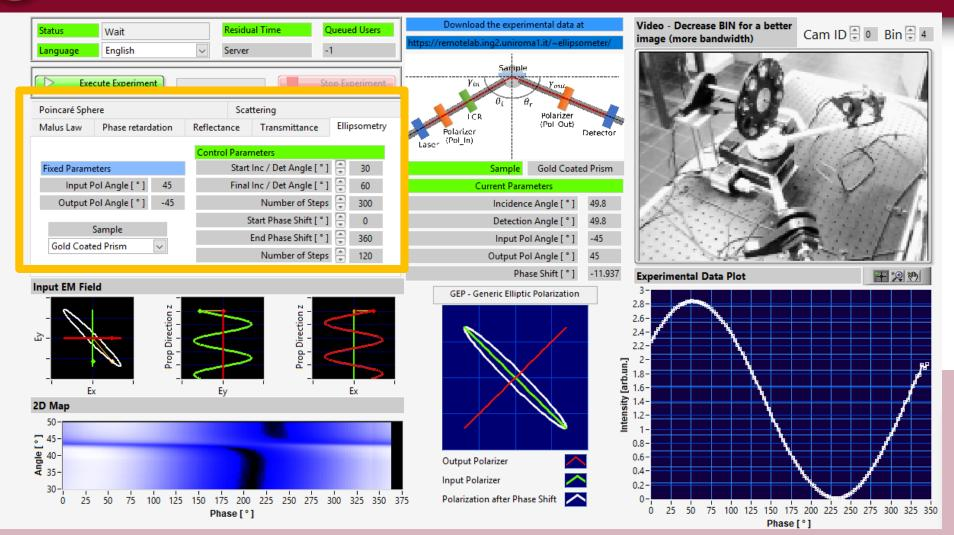
**Operation Mode Window** Permits to chose a specific operation mode and to input values of the parameters that can be controlled by the user
