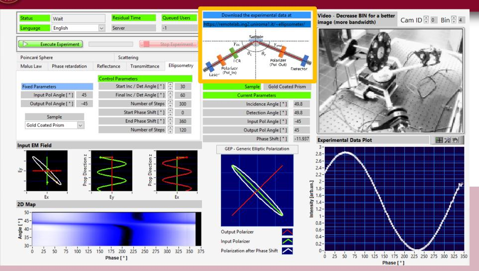
Setup Window Sketch of the optical layout and address of the remote directory where data can be downloaded by ftp by the user
