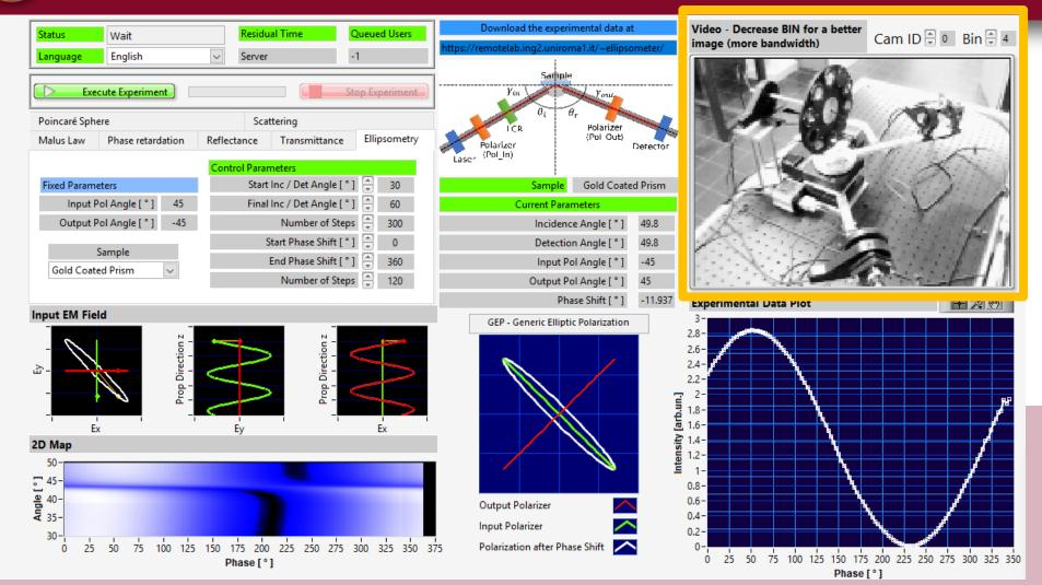
**Camera Window** Shows the real time conditions of the remote ellipsometer and permit to change binning to face bandwidth limitations
