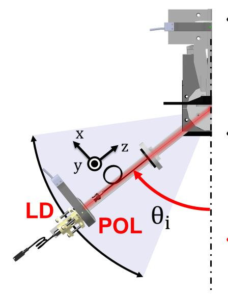
A polarized CW laser diode (LD) is used as illumination source:
