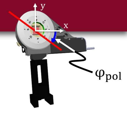
The linear polarization angle φ<sub>pol</sub> can be changed in the (0°, -90°) range with 0.001° resolution:
