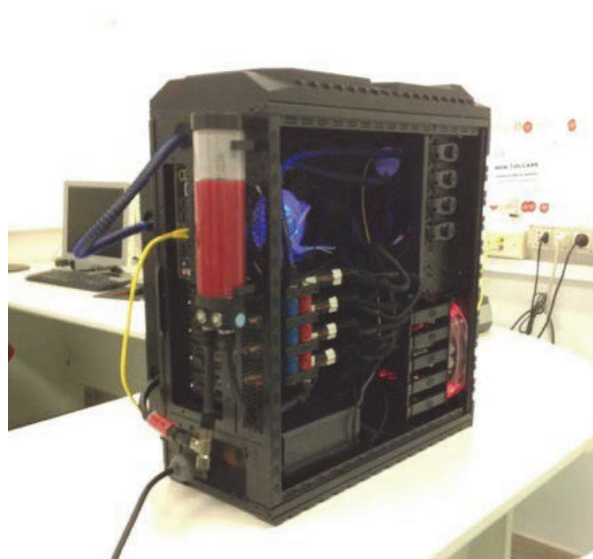
Figure 1: Closed circuit liquid cooled GPU server.
