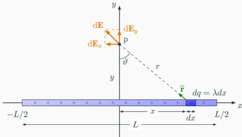
$$dE = K \frac{dq}{r^2} \Rightarrow dE_y = dE \cos \vartheta \Rightarrow dE_y = K \frac{\lambda dx}{x^2 + y^2} \frac{y}{\sqrt{x^2 + y^2}}$$
