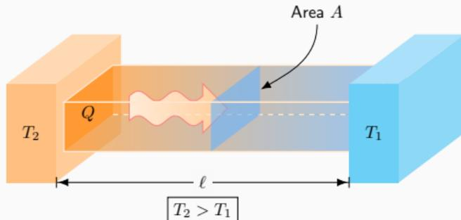
$$Q = K \frac{A(T_2 - T_1)}{\ell} \Delta t \Rightarrow \frac{Q}{\Delta t} = K \frac{A(T_2 - T_1)}{\ell}$$
