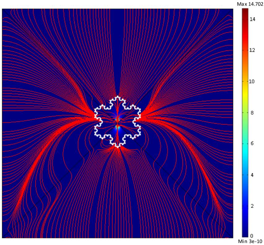
Figure 3.5: Heat flux streamlines at the stationary condition.
